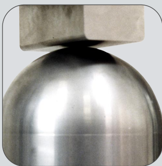
Flat rectangular striker with hemispherical anvil
